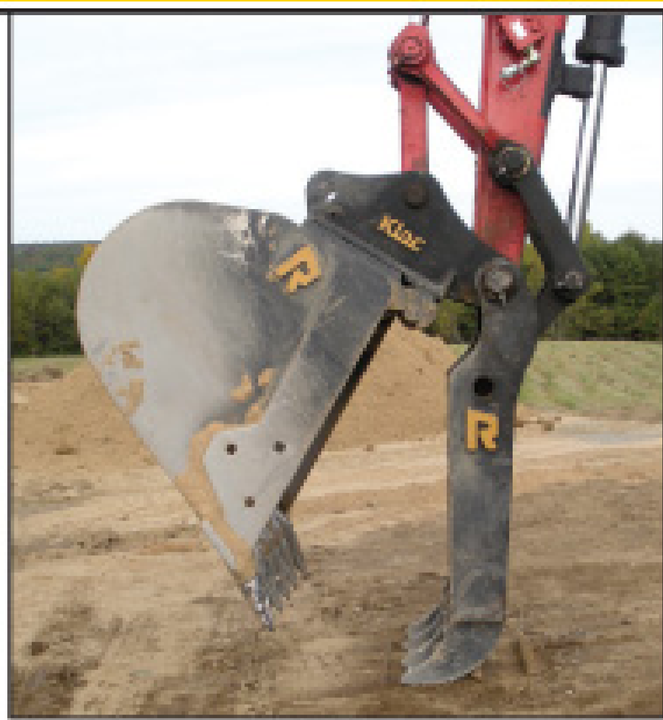
The Klac mechanical quick-coupler system from Rockland Manufacturing allows an excavator or backhoe operator to latch onto an attachment without leaving the cab.
