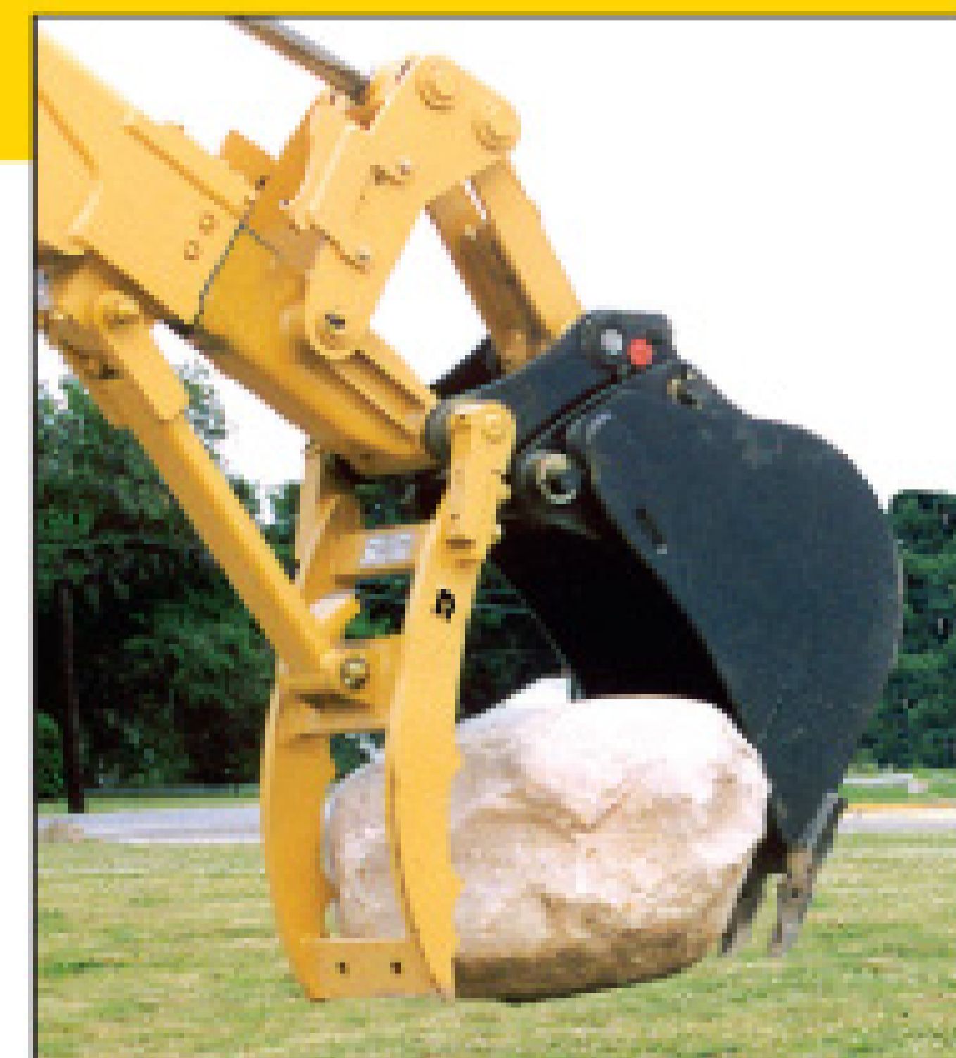
Designed for backhoes with extendible inner sticks, the hydraulically operated Smart Thumb from Rockland Manufacturing handles bulky objects and requires no additional hydraulic plumbing.
