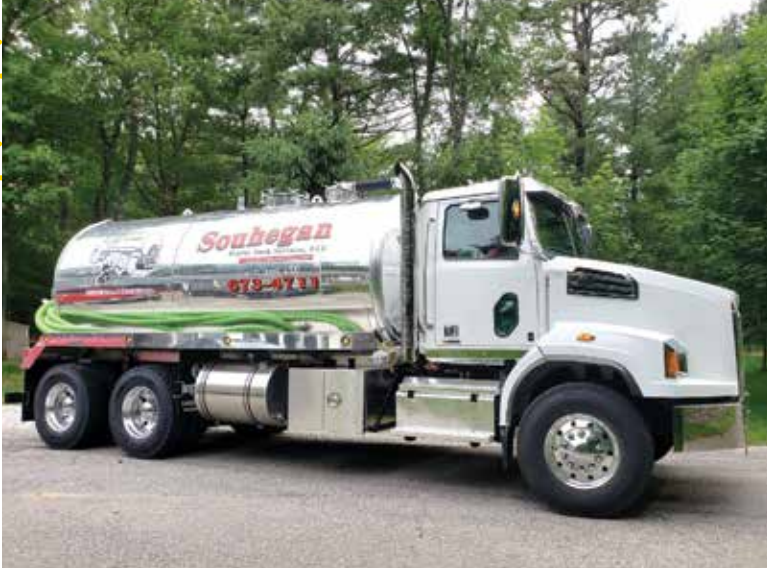
▲ Souhegan Septic Tank Service's 2023 Mack built out by Imperial Industries with a 4,250-gallon aluminum tank and National Vacuum Equipment 4310 blower.
